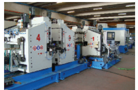
Right: Each head in the FPB features four servo-drive motors
